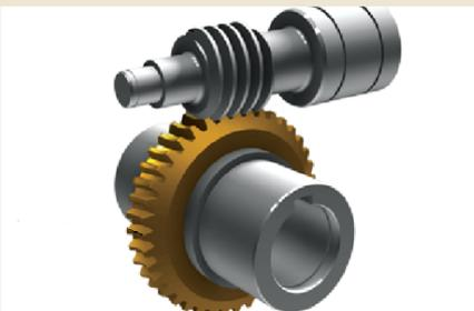
A worm drive is a gear arrangement that uses a worm (a gear in the form of a screw) and a worm wheel (which is similar in appearance to a spur gear). The two elements are also called the worm screw and worm gear. Worm drives are a compact means of substantially decreasing speed and increasing torque.
