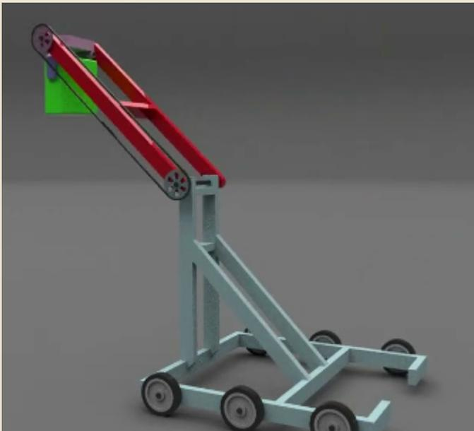
A virtual four bar uses chains/belts to create an effect similar to a four bar, where the end link/bar is kept at a fixed angle to the ground.
