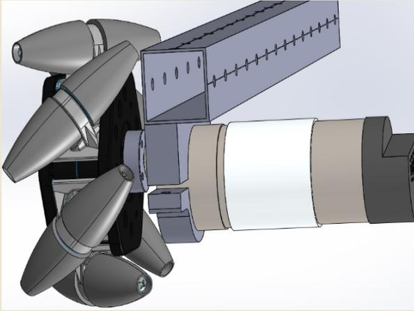
Direct drive consists in powering a mechanism directly from the motor axis. This way you put unnecessary load on the drive motor. This is because the shock loads can destroy gearboxes. Gearboxes are able to resist load along the axis of rotation for example when the wheel changes direction. However, in direct drive the gearbox shaft can be exposed to other shock loads outside of the normal axis for example when the wheel comes into contact with another robot.
