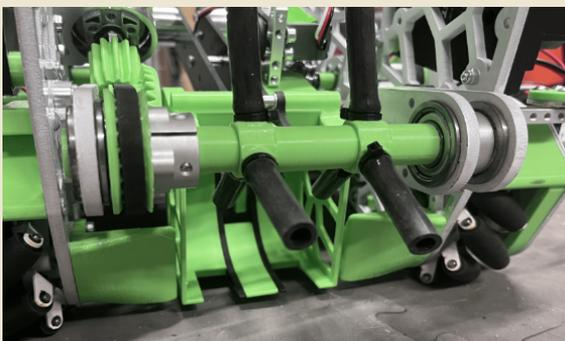
A direct transfer is the mechanism in which the items are moved to. It is placed behind whatever is picking up the game elements. It usually consists in an arm or a bucket to collect the items as soon as they enter the intake.
