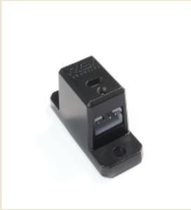
An Optical Time of Flight (ToF) Sensor is able to measure the distance between an object and the sensor. It does this by sending out a light beam and measuring the time it takes for the beam to travel to the object and back. Using this time and the known speed of light, the distance can be calculated. Be aware that the way the object interacts with light can change the accuracy of distance measurement.
