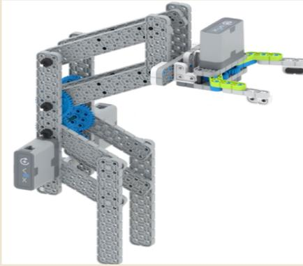
It is an extension of the four bar linkage because at the end of the four bar is mounted another one. This requires large space, but is a compact method of making large amounts of linear extension.
