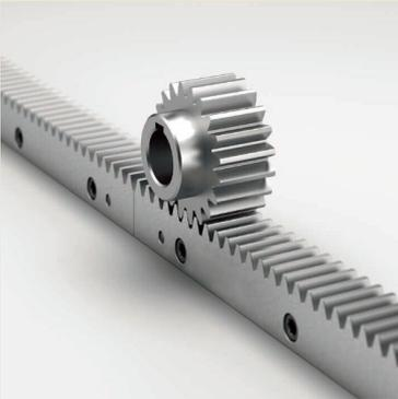
A rack and pinion comprises a circular gear (the pinion) engaging a linear gear (the rack). Together, they convert rotational motion into linear motion. Rotating the pinion causes the rack to be driven in a line. Conversely, moving the rack linearly will cause the pinion to rotate.
