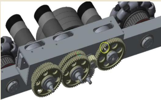
When you are meshing gears, you have to be sure that the gears are not too loose nor too tight. If the gears are too loose, the teeth will easily wear out, decreasing its longevity. But if they are too tight, they will have too much friction and possibly grind or bind up. **The ideal way to mesh gears is to make sure the teeth interlock and just touch the base of the gear.**
