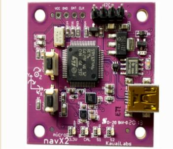
An Internal Measurement Unit (IMU) is a combination of a Gyroscope, Accelerometer, and Magnetometer. A Gyroscope is a device that reports the angular orientation of an object in 3 dimensions. An Accelerometer is a device that reports the acceleration of an object in 3 dimensions. Acceleration can be thought of as the rate of change of speed at any given instant. A Magnetometer is a device that measures the strength of magnetic fields in 3 axes.
